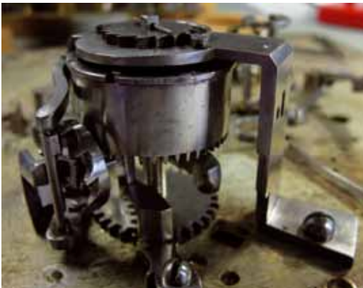
Fig. 15. Alarm mechanism. When the movement is assembled the whole alarm mechanism fits into the hours bell.
