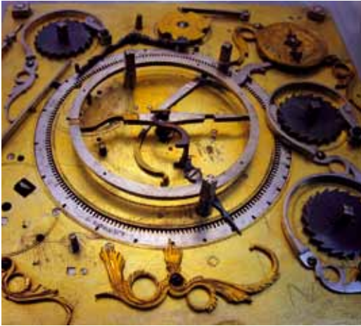
Fig. 17. Balance wheel. The bristle regulator was adapted to the balance spring.
