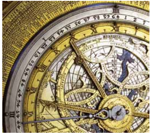
Fig. 5. Buschman clock, from the top to the bottom, steel minutes hand, moon phase and position, moon age and position of the sun, rete, dragon for the moon nodes.
